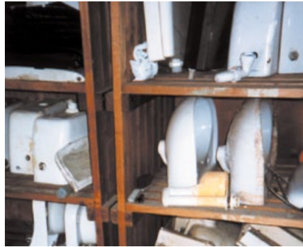
Figure 40 Asbestos-reinforced toilet cistern
