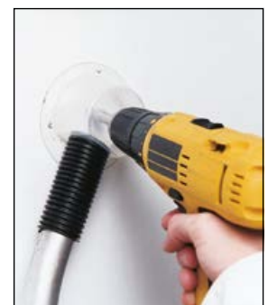
Control measures: shadow vacuuming and using a drill cowl as local extraction
