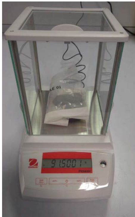
Figure A3.1 Water absorption sample being weighed
