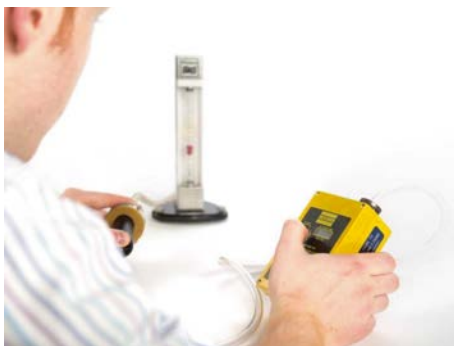
Figure A1.6 Flow rate of pump being measured
