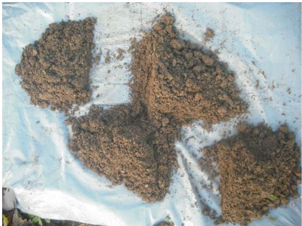
Figure A7.2 Example of coning and quartering: the two further quarters will be removed from the sheet
