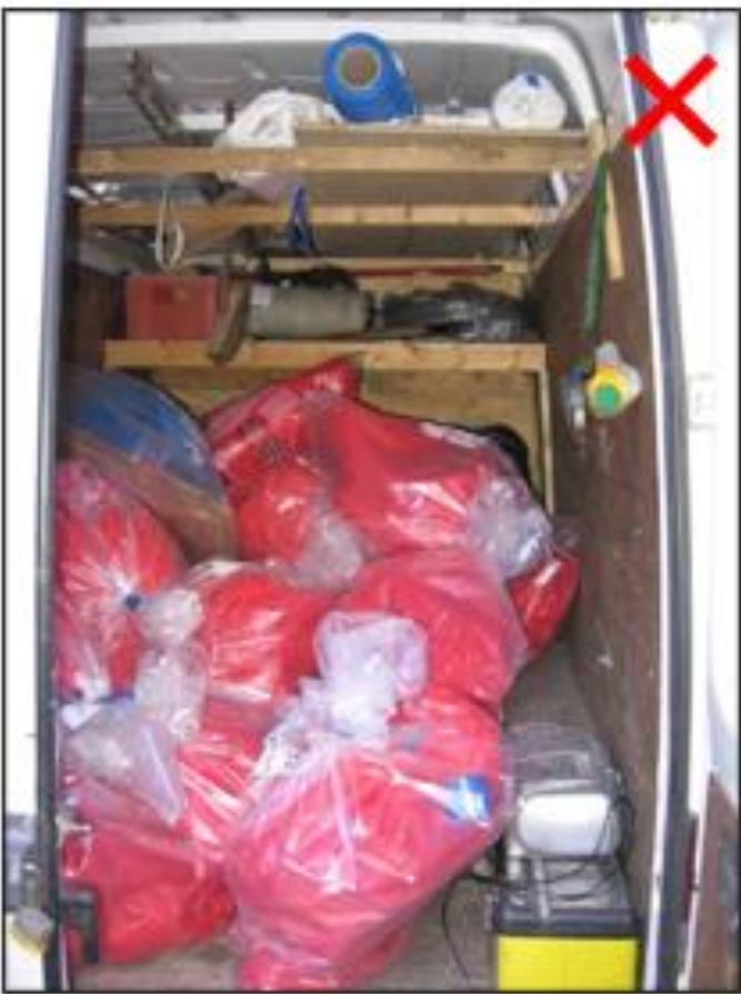
Why? The entire van appears to be dedicated to waste but there are other non-waste items carried in the same space which could fall onto the waste bags and split them open. If not stacked correctly bags could fall out on opening, or on closing, be damaged by entrapment in van door.
