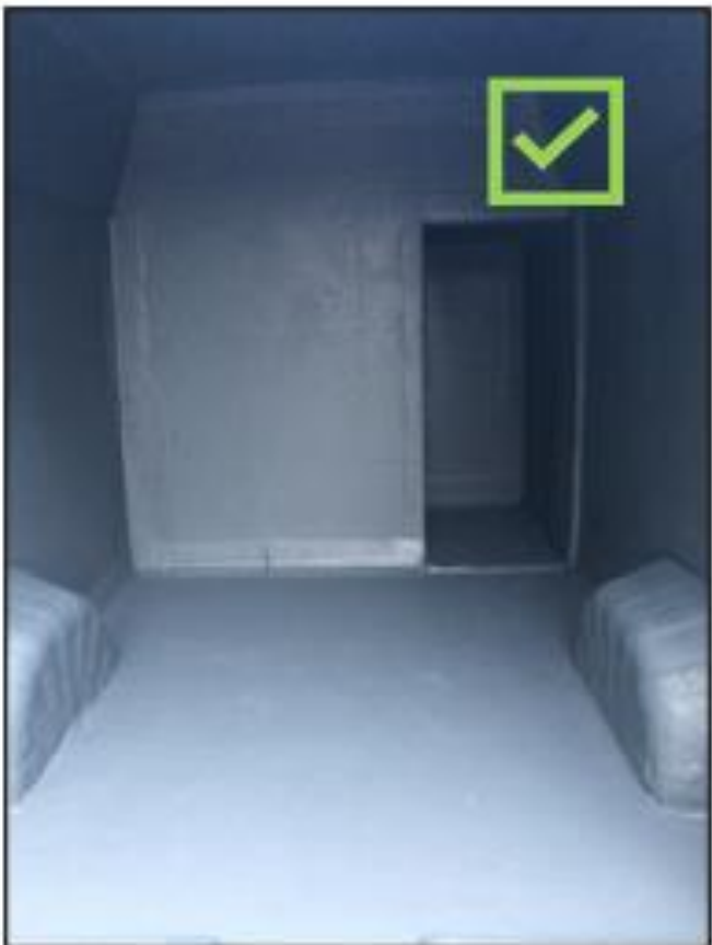
2. Entire van compartment sealed and segregated from top to bottom, rounded wheel arch edges to minimise risk of bag puncture [Not shown but there should be a secondary door to protect the door furniture, rear electrical lights and prevent waste falling out on opening]
